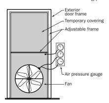
Testing the airtightness of a home using a variable speed fan called a blower door can help ensure that airsealing work is effective. Blower door testing is required by many energy efficiency certification programs. The test can usually be performed in less than an hour for simple floor plans and may be offered by utilities, weatherization agencies, and energy service companies.
