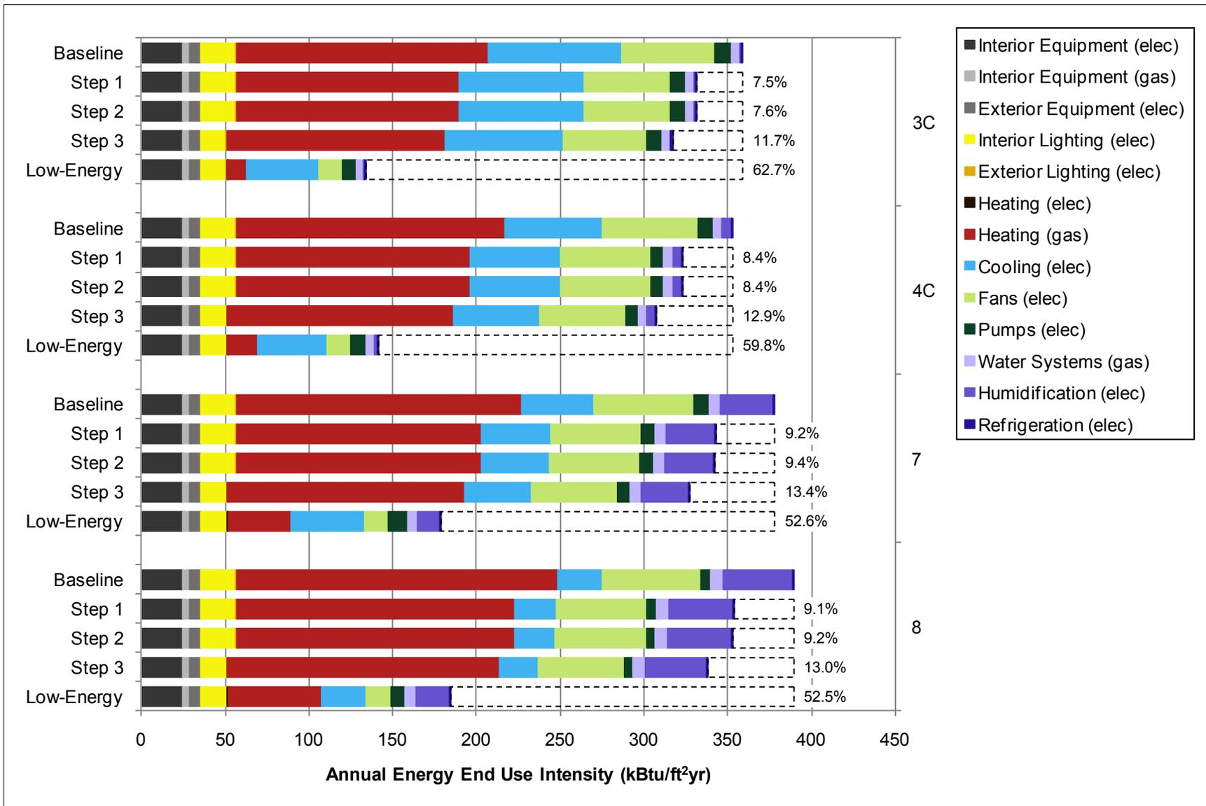
**Figure 5-4 Bundle analysis results for marine and cold climate zones**
