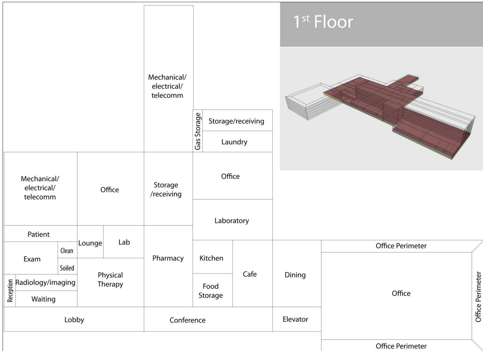
**Figure 3-2 Large hospital prototype first floor plan**
