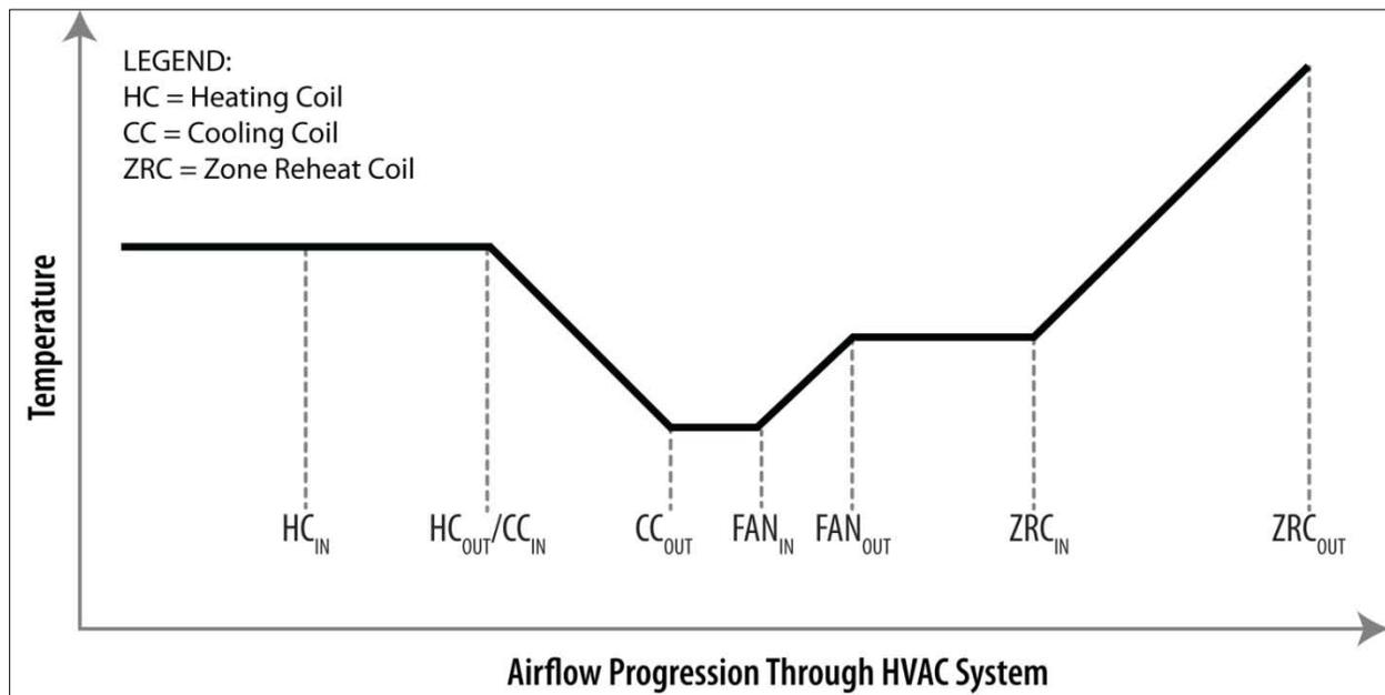
**Figure 4-1 HVAC system temperature diagram**
