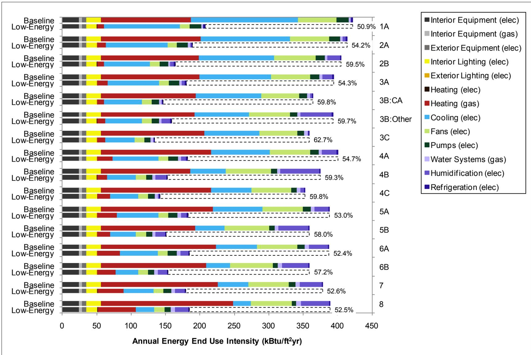
**Figure 5-1 EUI by end use for baseline and low-energy models**
