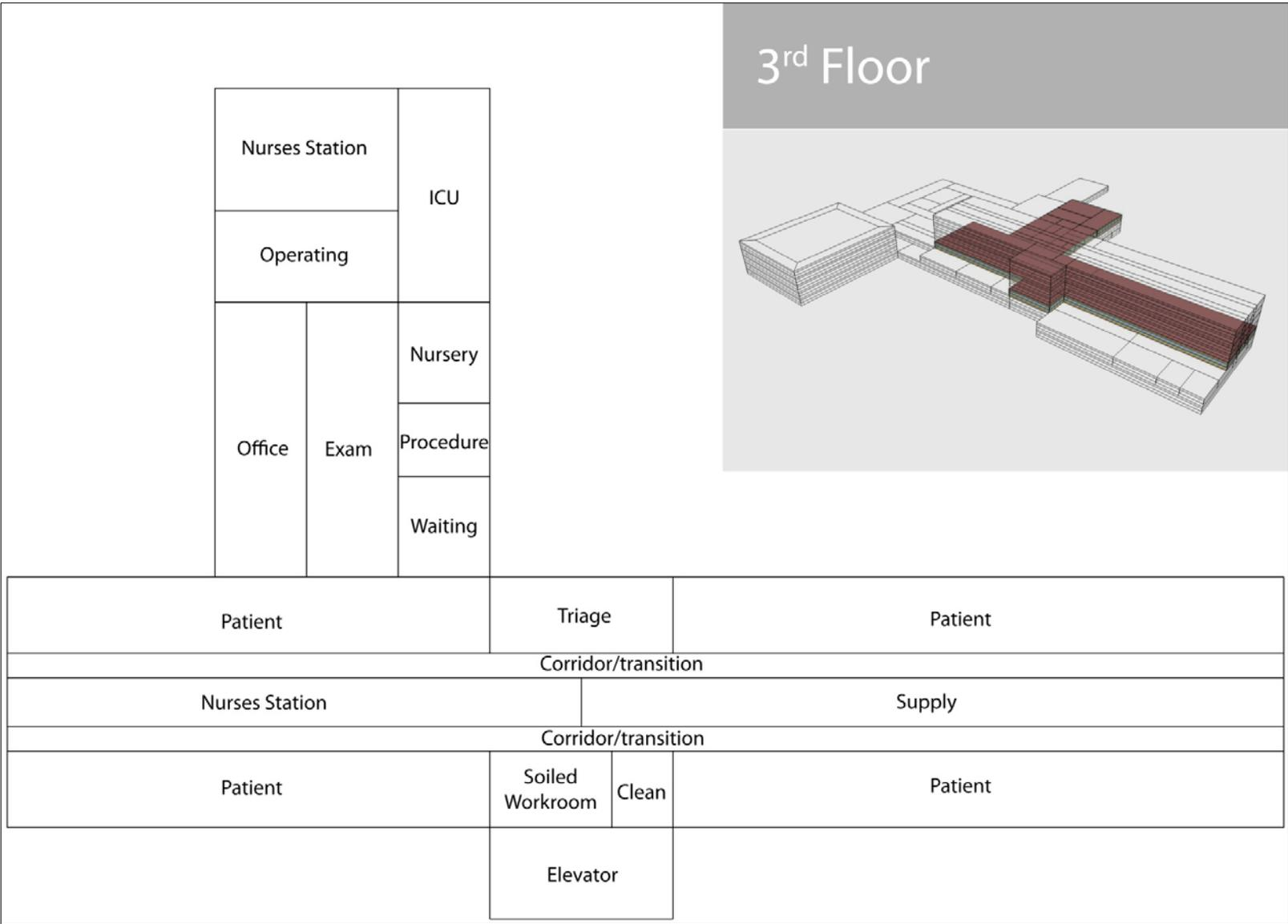
**Figure 3-4 Large hospital prototype third floor plan**
