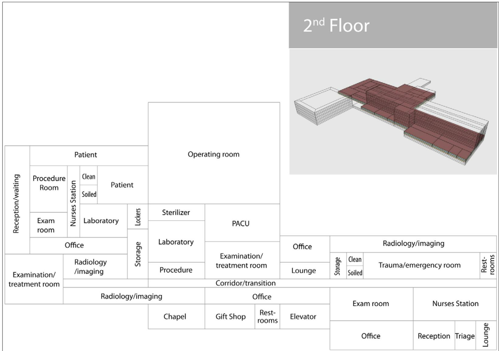
**Figure 3-3 Large hospital prototype second floor plan**
