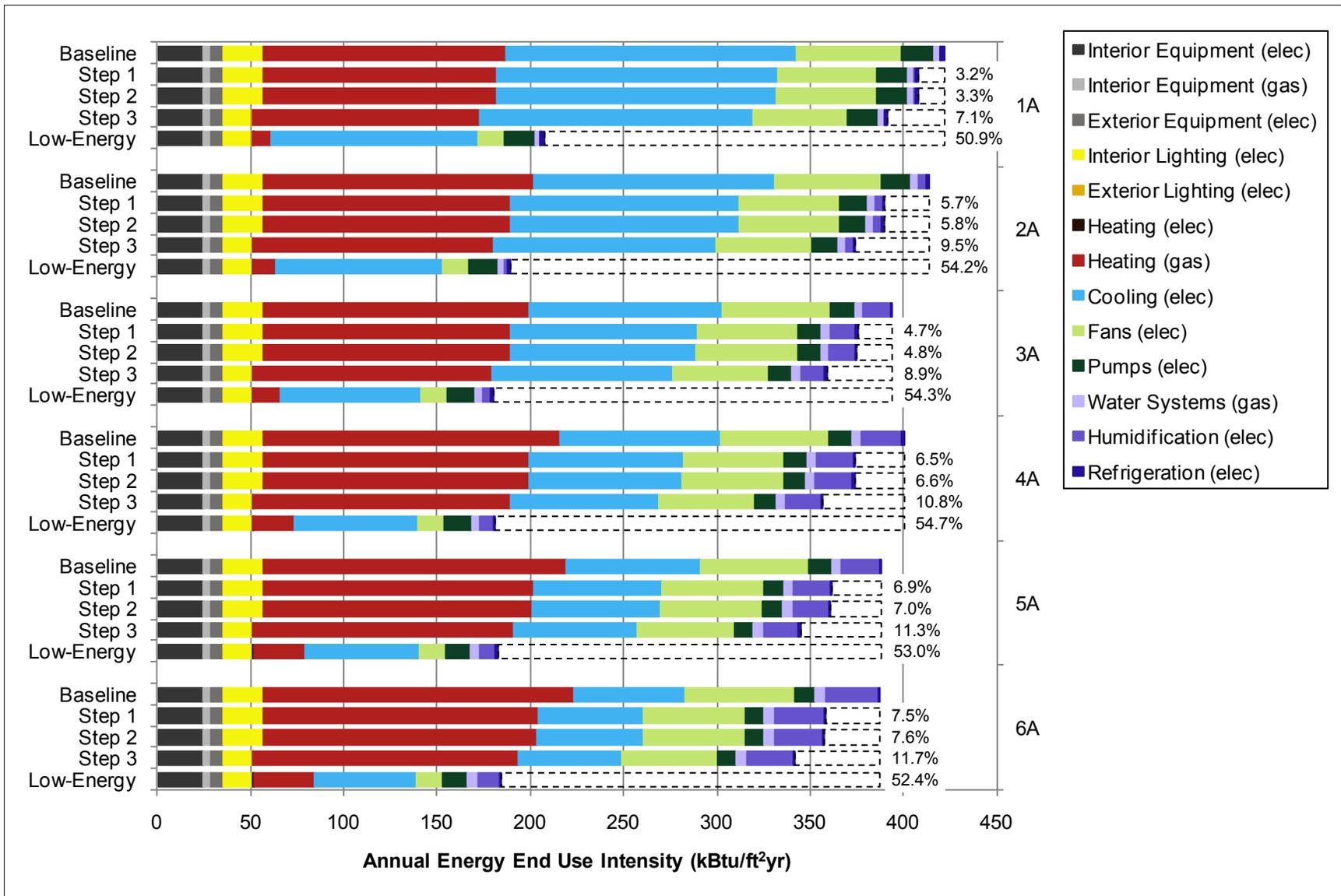
**Figure 5-2 Bundle analysis results for humid climate zones**
