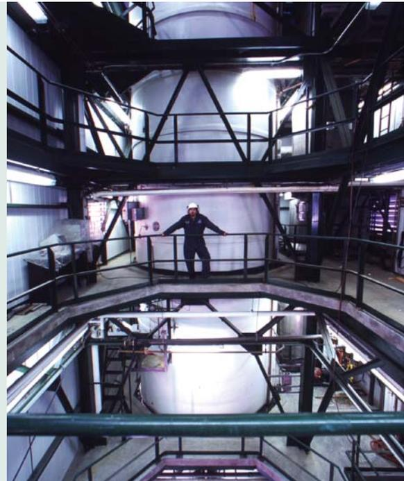
Fermenter at logen's test-scale cellulosic ethanol plant in Ontario, Canada. Credit: logen Corporation
